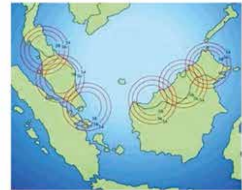
mSAT Coverage Spot Beams
